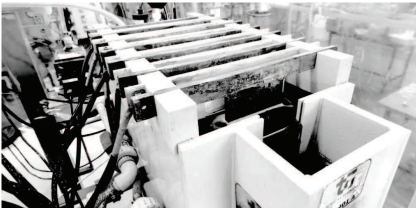
Electrowinning Pilot plant I and electrowon zinc plates at the TR technology centre.
