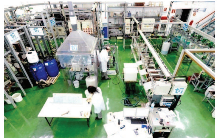
Pilot plant I at the TR technology centre. Pilot facilities for Leaching, Solvent extraction and Electrowinning
